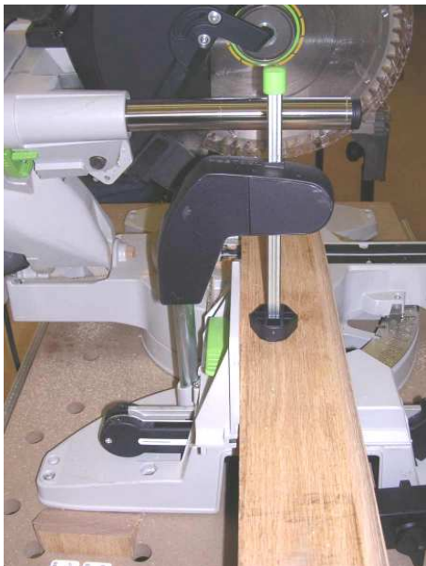
Hold down is typically robust and well engineered Festool. Note the miter gauge set jig in the storage compartment in the base sticking out to the lower left.
