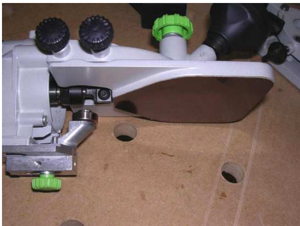
The right angle baseplate. The ball bearing rides the side and the adjustable depth bit trims laminate to the edge of the side. Again, infinitely adjustable in a very fine tune manner and offset plate for stability.
