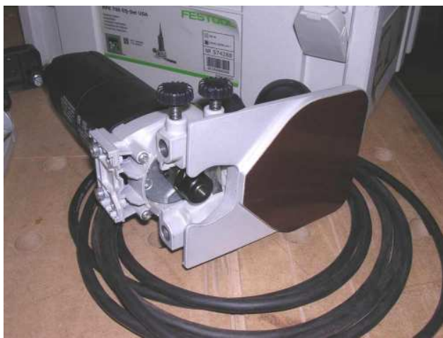
Standard mount laminate trimmer. But it has fine tuning controls, great stability, offset baseplate, many other features. This does conventional laminate trimming to the edge of the top.
