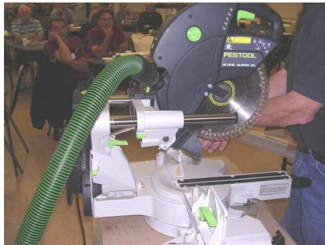
Note that when the saw is set up on chop box mode, the setup takes advantage of the height of the space to the rear of the blade to allow a very deep cut.
