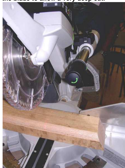
The tilt is controlled by a flip lock in the rear and a front handle twist. Set it, flip the lock again. Front tilt controls make it easier to get where you want without going to the back of the saw.
