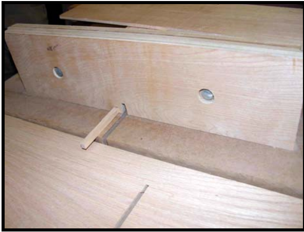
Finger joint jig. Note indexing pin.
