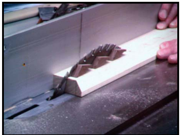
3 drawer pulls on a form being side beveled.
