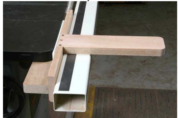
This little jig supports the sled on the working side of the saw. If you have a good fence like a Beisemeyer!
