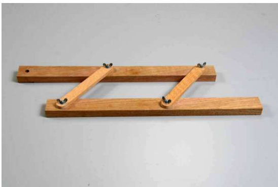
Cove cutting jig for cutting coves on a table saw. This is a very simple, very cool device that allows you to make a wide variety of coves in the table saw.
