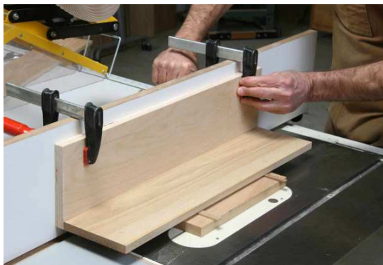
Pattern Cutting Jig. See text.
