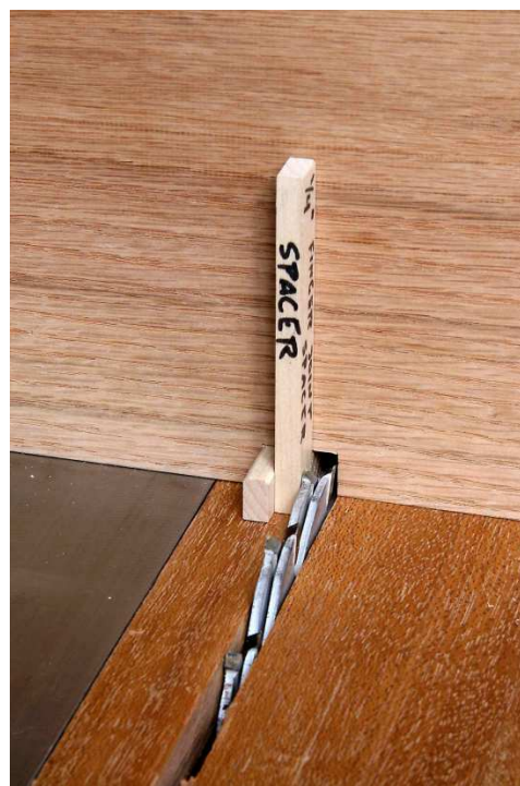
The indexing pin in place, use the remained of the indexing pin stock as a spacer to make the next hole. You will need this spacer in making finger joints – one side is offset from the other.
