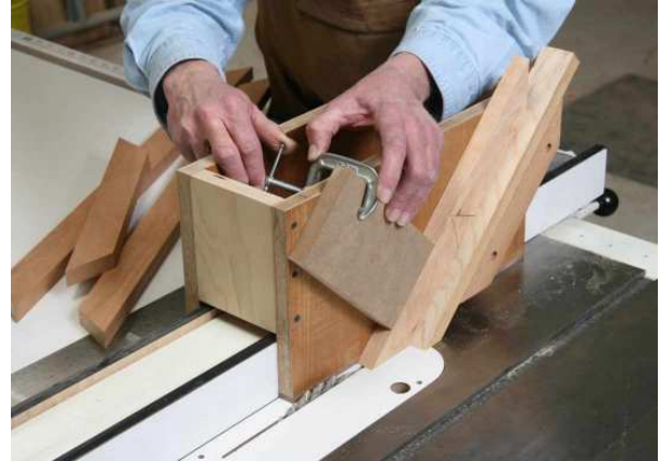
The other side of the jig. Sort of “PUSHING” the piece through the blade.
