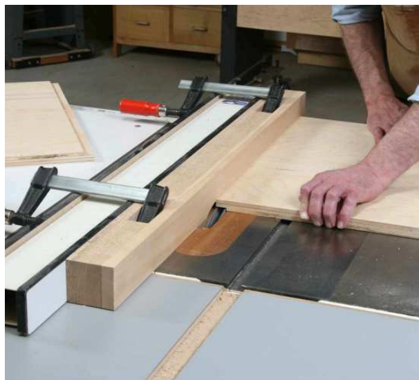
This sacrificial fence keeps the clamps out of the way.
