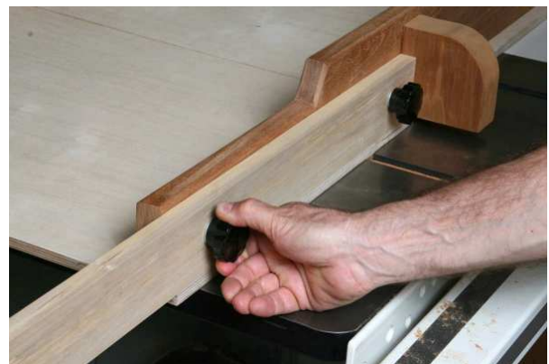
The extension arm fits on with readily available threaded knobs. Note the rear piece of mahogany – THIS IS NOT A PUSH HANDLE – I originally said it was and should have known better – Paul quickly corrected me – HANDS do not go IN LINE with the blade, RIGHT? It is purely a blade guard. Not seen in other jigs of this type.
