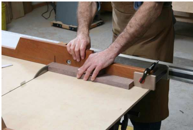
The crosscut sled in use with a stop block. Note Paul's hand position – not in line with blade.
