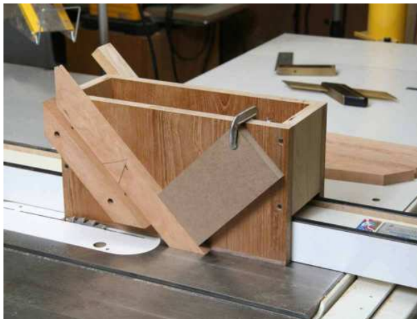
Tongued miter jig in action with hold down. Sort if “pulling” the piece through the blade.....
