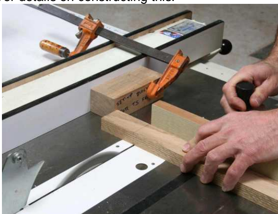
Standoff clamped to the fence. It is a block of wood. Even I can make this.
