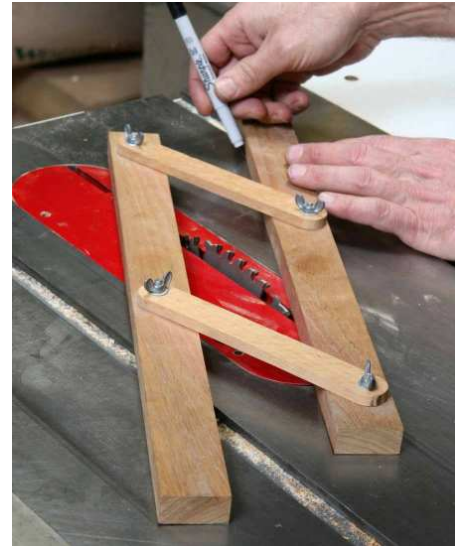
Setting the width of the cove. From the stock. Mark the table with pencil.
