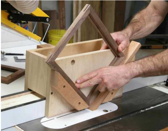
Making a strong picture frame is easy with this jig. Note the tenoning jig is on the other side! Also notice there are holes in the box. These are used as screwdriver access to mount the vertical member of the tenoning jig.
