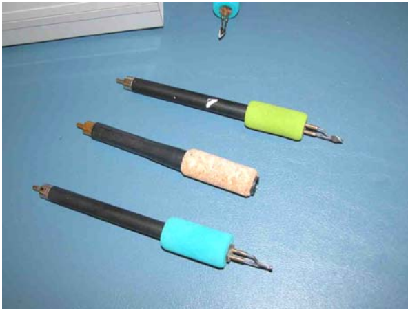
The pens at the top and bottom are Optima one piece pens and the thing in between them is a Colmar pen handle. Typically, you buy the burner base, a cord and a pen or a pen handle and tips.
