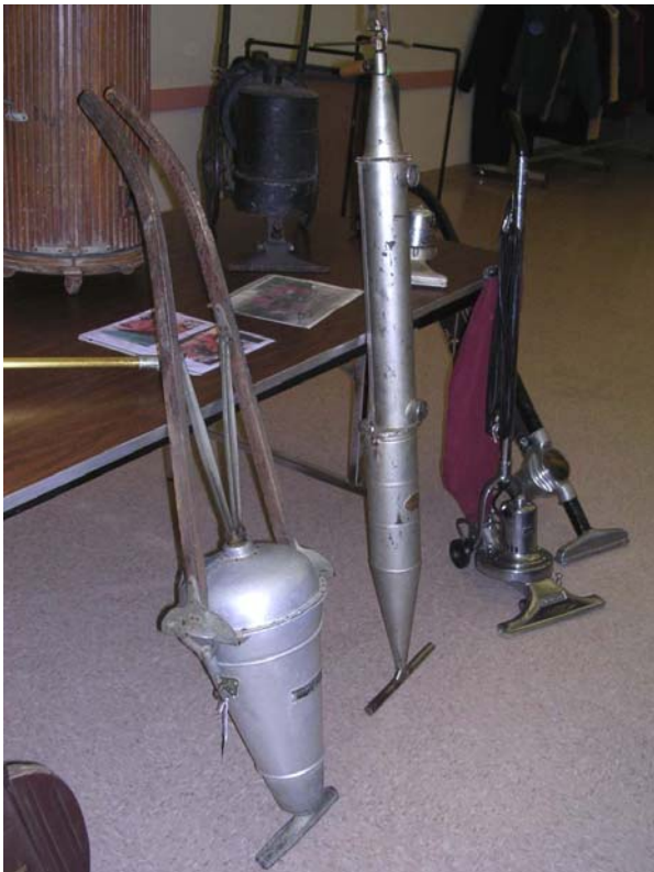
OK, we have a hybrid pumper style, a plunger style, and an early electric model here, left to right.
