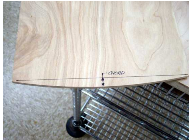
This is what Craig means by a cambered edge. The size of the chord will determine the "Scalloped" effect.
