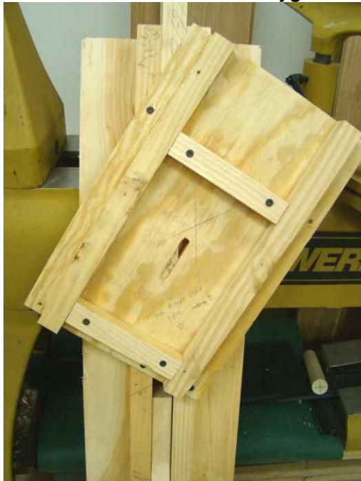
Jig itself cut to fit router base and it just slides in the groove. Tile it the other way to do the other shutter stile.
