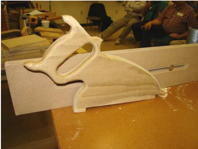
Another style of push stick. Common features are a little push edge in back and a flat surface that acts to hold down work.
