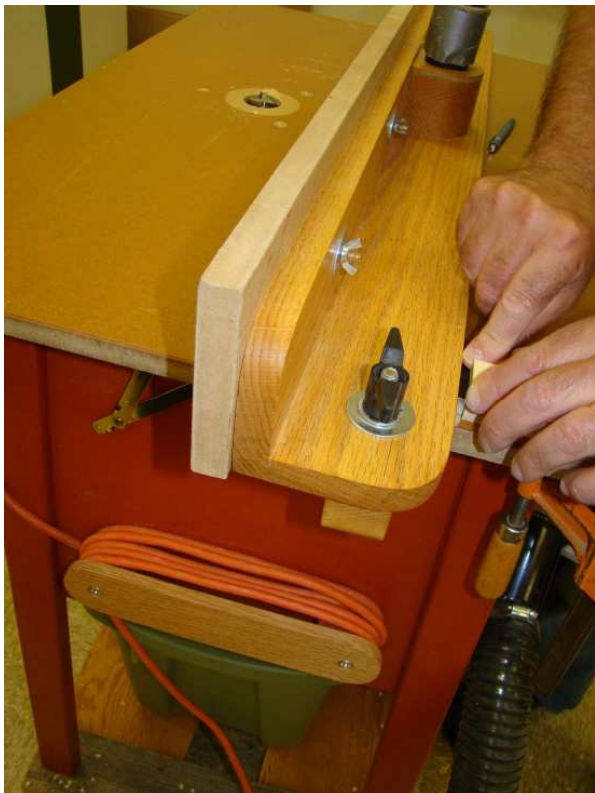
Decent shot of Bill's fence. Oak butt joint frame with MDF split fence face. Common hardware. Here, Bill is clamping on a micro adjust.
